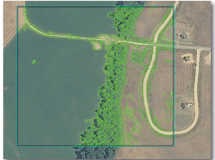
Figure 3: NAIP Imagery was segmented into polygons by grouping pixels with similar spectral characteristics.
